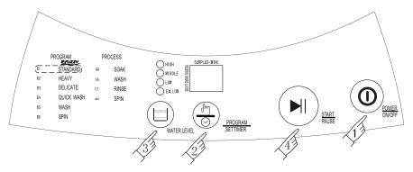
1 Press the "POWER ON/OFF" button to switch on the power supply
